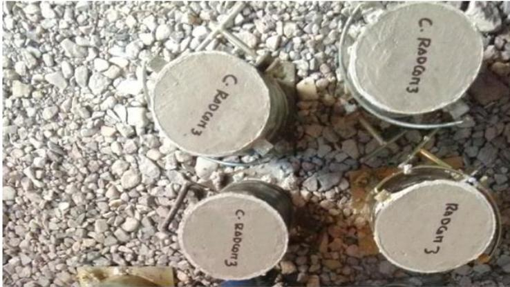
Figura 51. CR3 – Probetas de concreto  $f'c=210.00$  kg/cm<sup>2</sup>
