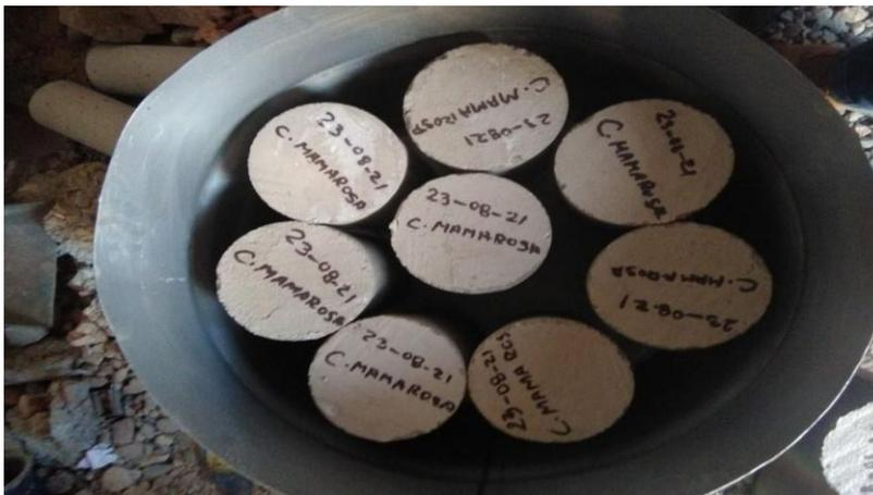
*Figura 50. CMR – Probetas de concreto  $f'c=210.00$  kg/cm<sup>2</sup>*
