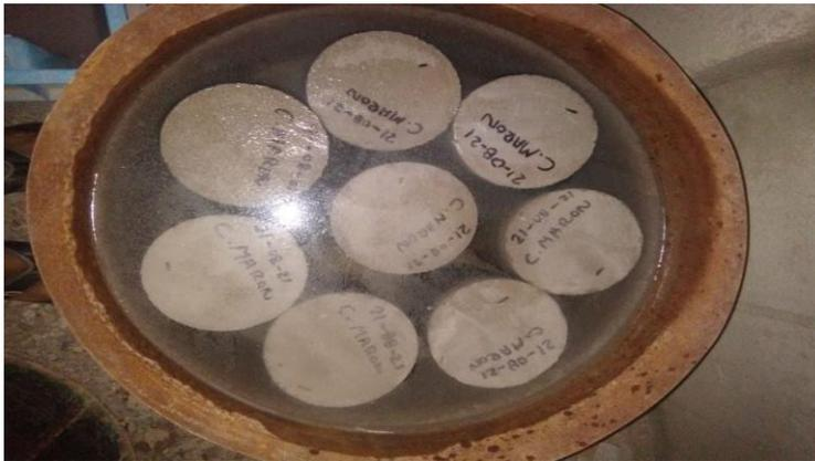
*Figura 52. CM – Probetas de concreto  $f'c=210.00$  kg/cm<sup>2</sup>*
